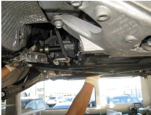
Figure 2. Supporting the flange shaft.
