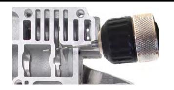
**Step 2** Lube and converter flow: Drill a 3/64" (.042 - .047) hole sideways through this wall about an 1/8" down from the top.
