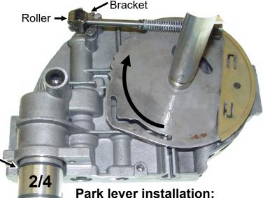
While rotating detent plate in direction of arrow hook roller
