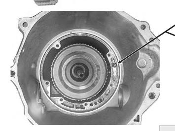
If the case has a 2" deep hole here it MUST HAVE a cooler bypass valve installed. Less than 1" no bypass valve.
