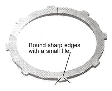
1st & 2nd type UD/OD pressure plates are flat & sharp across top and tooth. File teeth edges. Just barely file edge of teeth so sharp edge won't cut snap ring.
