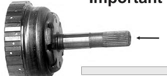
Drill cup plug in underdrive hub .086 to .096 to increase lube flow to the planets.
