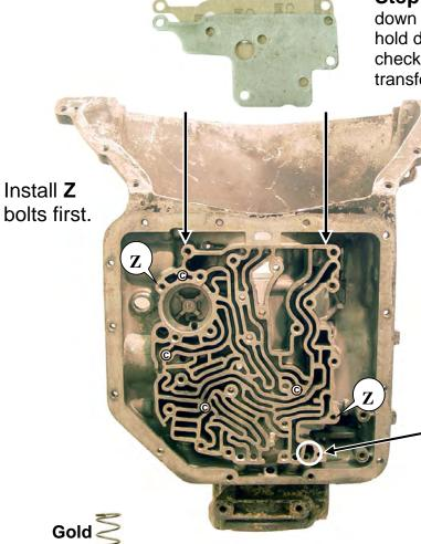
**Step1.** New special gasket under hold down plate stops high clutch failure. Install hold down plate and gasket after installing checkballs and TransGo® plate with welded transfer plate.
