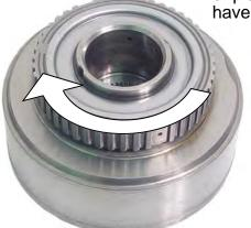
Intermediate Sprag Outer race must freewheel as shown
