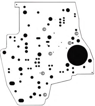
New SK<sup>®</sup> plate produces short smooth shifts. This product is not for making firm Hi-Perf type of shifts. If you want firm shifts and complete gear control order TransGo Reprogramming Kit.
