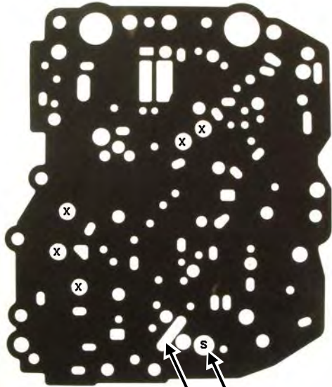
Manual Gasket Has Slot & Hole at "s".
